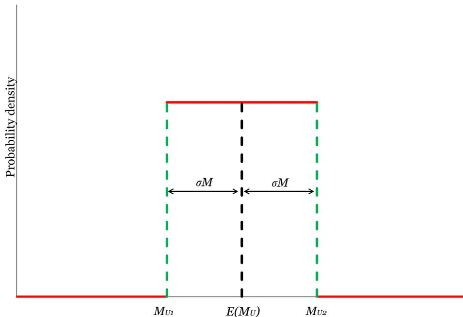
Figure 2-1 Probability density function of the  $M_U$  value
