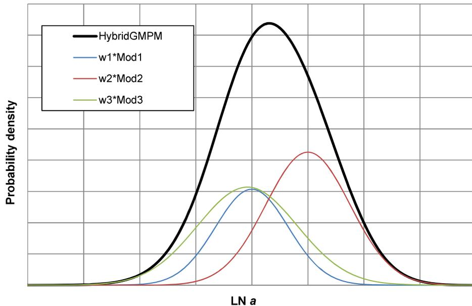
Figure 2-21 Example of a hybrid GMPE
