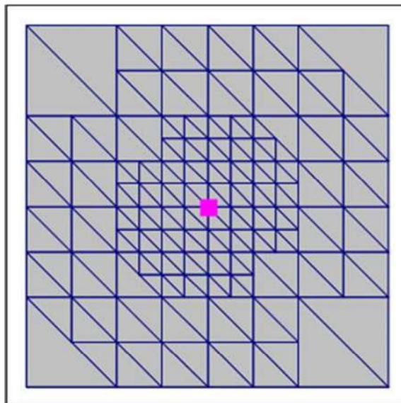
**Figure 2-24 Source subdivision with minimum triangle size=5km,
