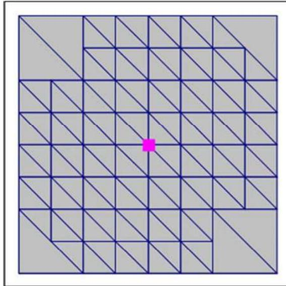
**Figure 2-23 Source subdivision with minimum triangle size=11km,
