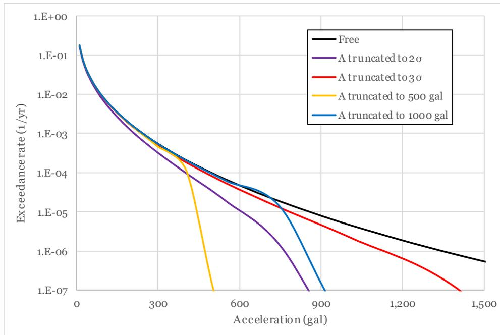
**Figure 2-20 Effect of different truncation schemes on GMPM**
